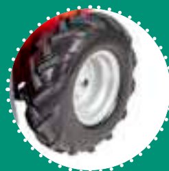
DRIVEN WHEELS puncture proof 13x5.00-6"
